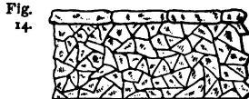
Fig. 14. Rustic or Rag. —Stones of irregular form, and dressed to make close joints.
